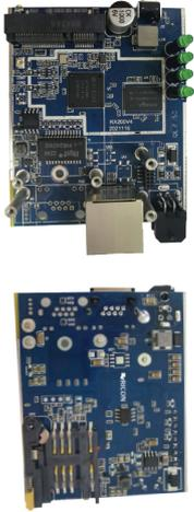
**RICON P9922MC PCBA Integrated Router**, by Ricon Mobile Inc. industrial grade quality, designed and manufactured in accordance with 3G/LTE cellular network technology to be integrated inside any electronic hardware needs wireless connectivity. With the embedded cellular module, it is widely used in many cases such as ATM connection, remote office security connection, data collection etc.
