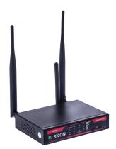
**RICON S9922M2E-LTE Router** by Ricon Mobile Inc. industrial grade quality, designed and manufactured in accordance with 3G/LTE cellular network technology. With embedded cellular module, it is widely used in many cases such as ATM connection, remote office security connection, data collection etc.
